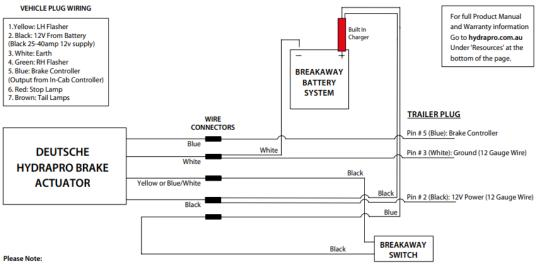
1. Vehicle wiring for Black, White, and Blue must be wired as stated for the unit to operate correctly.
