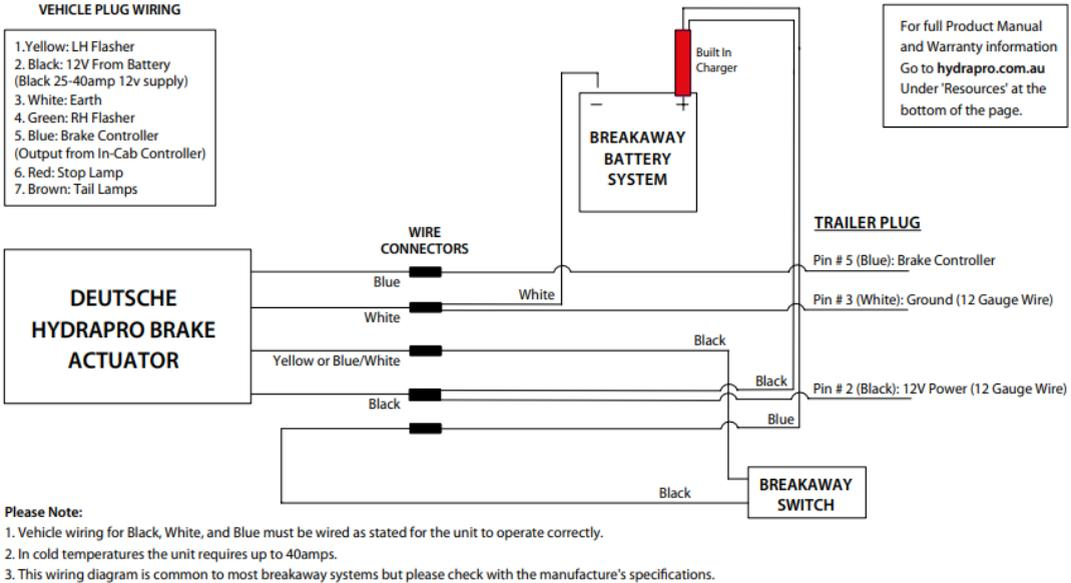
It is important that the Black Power and the White Ground wires from the tow vehicle to the actuator unit are the correct size (12 gauge wire minimum) and properly terminated to a 25-40 amp circuit on the vehicle. For best performance, use 10 gauge wire.
